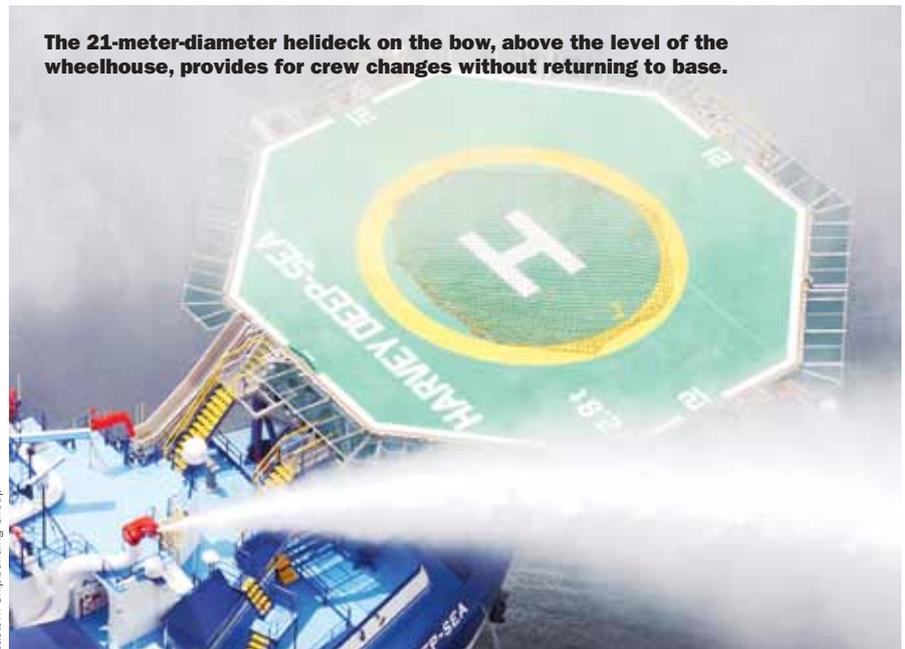
The 21-meter-diameter helideck on the bow, above the level of the wheelhouse, provides for crew changes without returning to base.
