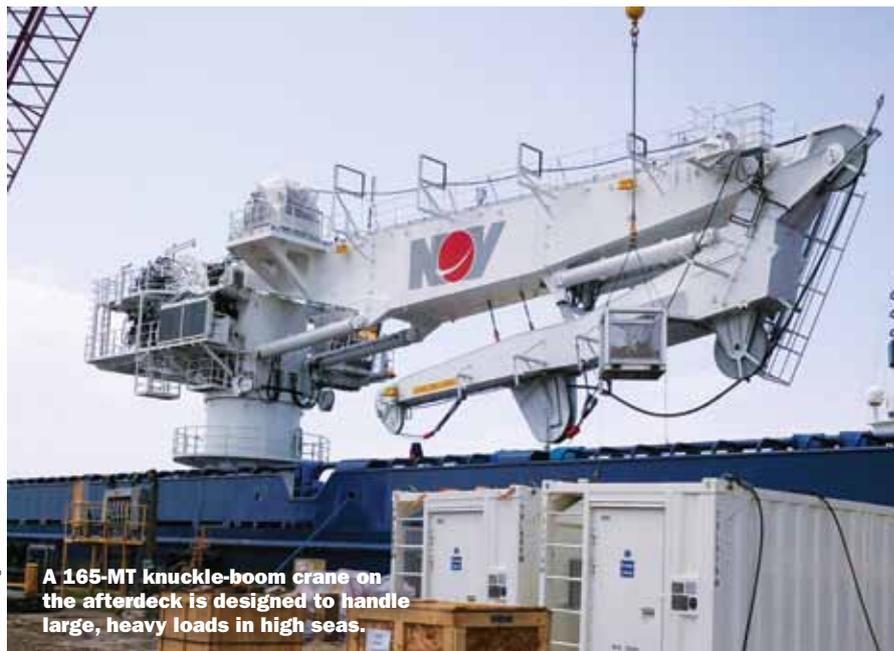
**A 165-MT knuckle-boom crane on the afterdeck is designed to handle large, heavy loads in high seas.**
