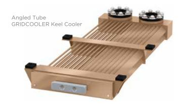
ILLUSTRATION: Angled Tube GRIDCOOLER Keel Cooler The angled tube GRIDCOOLER Keel Cooler's tubes are positioned to enhance and exploit the natural convection current generated by the heat exchanger.
