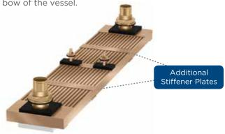
**L SERIES** support plates are designed to minimize intermediate support bolt hull penetrations. These support plates extend beyond the keel cooler side tubes, providing additional securing options. This feature is especially useful in retrofitting a keel cooler to an existing vessel.
