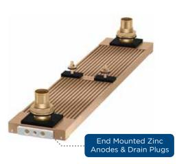
**HD SERIES** stiffener plates can be added to units providing additional support to prevent tubes from bowing, bending, or vibrating from the impact of heavy seas. These plates do not have additional mounting points. The HD Series is ideally suited for applications where the vessel is operating in heavy pounding seas, strong currents, or the keel cooler is positioned near the bow of the vessel.
